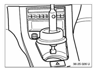
Pull rubber grommet out of body opening and remove upwards together with shift lever.
