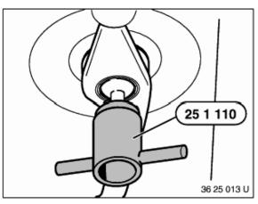
Fit special tool 25 1 110 and rotate counter-clockwise through 90°.
