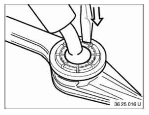
Press down on bearing shell at point of retaining tabs until they are heard to engage.
