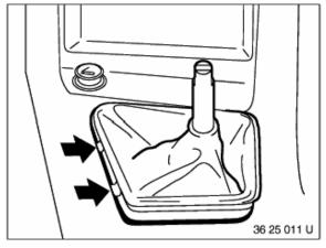
Lift and pull cover off shift lever. Remove foam rubber cover (if fitted).
